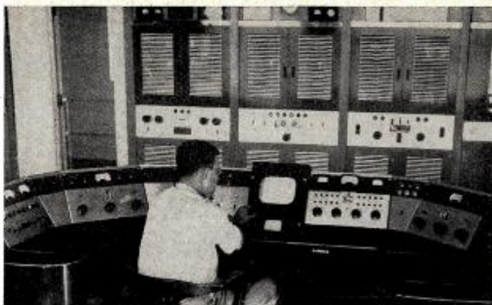
THIS COMBINATION console arrangement has been installed by WKY-TV Oklahoma City, which will begin commercial operations by mid-May or early June, according to P. A. Sugg, station manager. Console enables an engineer to control the television, FM, AM and auxiliary broadcast signals. Horace Merriman, transmitter supervisor, is testing the television monitor and controls in the center of the board. At left are the auxiliary transmitter controls. FM operations are at the right of the panel. Ninety percent of the TV transmitter installation is now complete.
